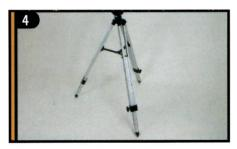
All three legs should be the same length to provide a level platform for the telescope.
