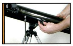
Secure the tube to the mount using the two threaded mounting bolts. Tighten to secure in place.
