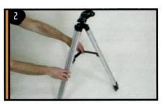
To set up the tripod, spread the legs outward until they are fully extended and push down center locking brace.
