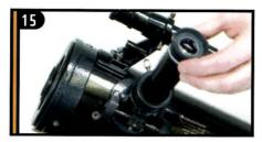
Insert the barrel of the 20mm eyepiece into the focuser and tighten the set screws.
