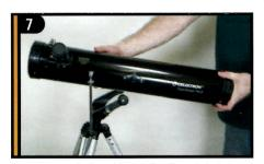
Locate the optical tube and line up the tube with the holes on the mount.
