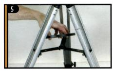
Place the accessory tray on top of tripod's center leg brace. Thread the tray into the threaded hole in the center of the leg brace.
