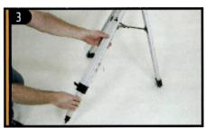
Extend the center portion of each of the three tripod legs down 6-12". Use the three tightening screws located at the bottom of each leg to secure the extended legs in place.
