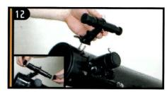
Orient the finderscope so that the lens window is facing towards the front of the tube. Place finderscope over the posts on the tube and replace knurled nuts.
