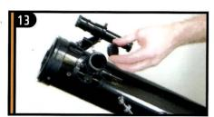
Loosen the set screws on the focuser so that they do not obstruct the inner diameter of the focuser. Remove the plastic cap covering the end of the focuser.
