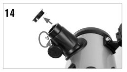
Loosen the setscrews on the telescope focuser and remove the dust cap.
