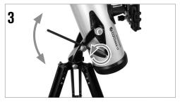
To move the telescope up and down, hold the focuser of the telescope in one hand and loosen the knob on the slow motion rod guide. The telescope can now be moved up or down as desired. When you are close to your target, tighten the knob to secure the telescope in place.
