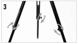
Extend the center portion of each of the three tripod legs down about 6 to 12 inches. Use the tightening screw on each leg to secure the extended leg in
