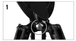
To move the mount left and right, loosen the azimuth tension knob located on the yoke mount between two of the tripod legs.
