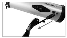
Slide the altitude rod on the into the rod guide on the mount and lower the altitude hubs on the telescope tube into the cradles on the top of each yoke arm.
