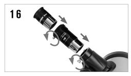
To use the Barlow lens, remove your eyepiece from the telescope focuser, insert the Barlow lens into the focuser and insert your eyepiece into the Barlow lens. This will double the magnification of whatever eyepiece you use it with.
