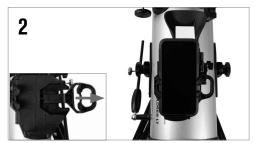
Pull open the spring-loaded slider on the top of the phone dock and set the phone into the holder so it is flush with the bottom lip of the phone holder. Slowly release the slider to secure the phone in place.
