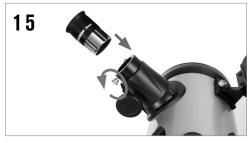
To install the eyepiece, loosen the setscrews on the focuser. Insert the silver barrel on the bottom of the eyepiece into the focuser and secure by tightening the setscrews. Always start using your low-power eyepiece (25 mm) to help you find the target you wish to view. You can always change to your high-power eyepiece (10 mm) later.
